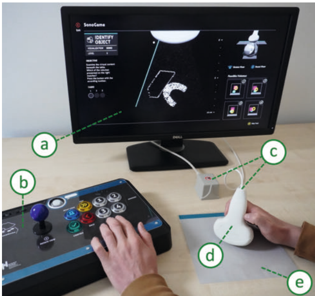
► Fig. 3 Overview of the SonoGame setup. a: game screen, b: game controller, c: motion tracking system, d: 3D-printed probe, e: marker indicating the surface of the examination volume.
